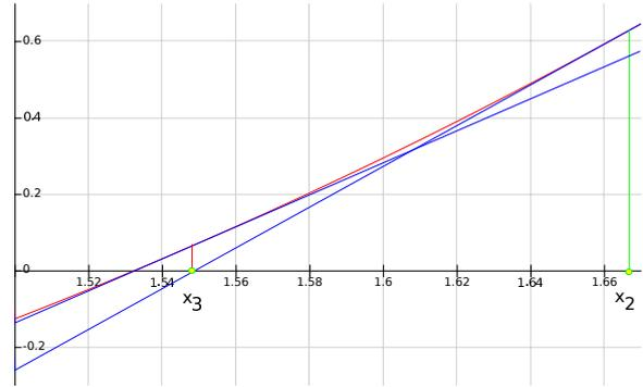
The equation  $x^3 - 3x + 1 = 0$  has three roots. We can use Newton's method to determine the approximate value of the 3 roots. We take initial guesses of 2 and 0.5 and  $-2.5$ . We get:
