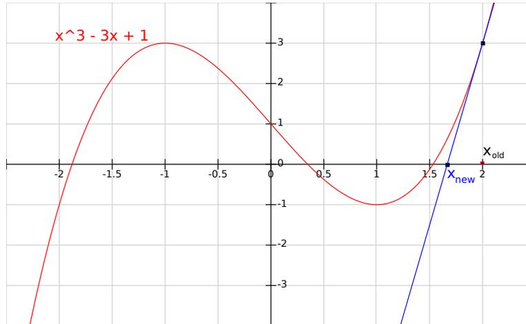
Newton's method is to take a guess for the root – we take  $x_{\text{old}} = 2$ . If the guess is not a root, then follow the tangent line at  $P = (x_{\text{old}}, f(x_{\text{old}}))$  to where it crosses the x-axis and call that point  $x_{\text{new}}$ .
