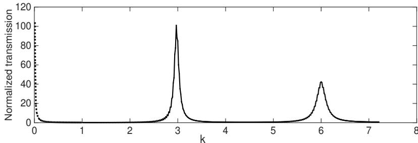
FIG. 1.2. Normalized transmission with  $\varepsilon = 0.02$  and  $\ell = 1$ . The normalized transmission is defined by  $P/P_{inc}$ , where  $P$  and  $P_{inc}$  denotes the transmission power and the incident power over the lower slit aperture respectively.
