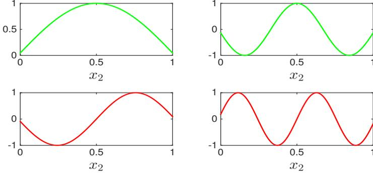
FIG. 5.1. The shape of the leading term along  $x_2$  for the first two odd resonant modes (Top) and the first two even resonant modes (Bottom) when  $\varepsilon = 0.01$ . It is calculated that the first two odd resonant frequencies are  $k_{1,1} \approx 3.05$  and  $k_{2,1} \approx 9.15$ , and the first two even resonant frequencies are  $k_{1,2} \approx 6.10$  and  $k_{2,2} \approx 12.20$ . Note that the leading term of resonant modes are constant along the  $x_1$  direction.
