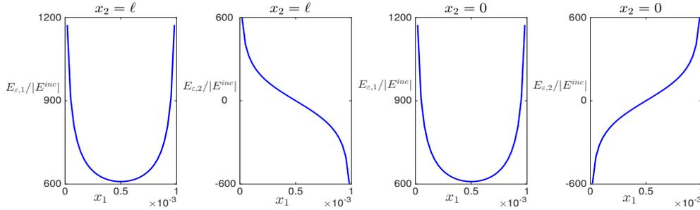
FIG. 6.2.  $E_{\varepsilon,1}/|E^{inc}|$  and  $E_{\varepsilon,2}/|E^{inc}|$  on the upper and lower gap apertures when  $k = 0.1$ ,  $\ell = 0.01$ , and  $\varepsilon = 0.001$ .  $E^{inc}$  is the incident electric field. It is seen that  $E_{\varepsilon,1}(x_1, \ell) = E_{\varepsilon,1}(x_1, 0)$  and  $E_{\varepsilon,2}(x_1, \ell) = -E_{\varepsilon,2}(x_1, 0)$ . This is consistent with the asymptotic expansions in Theorem 6.3.
