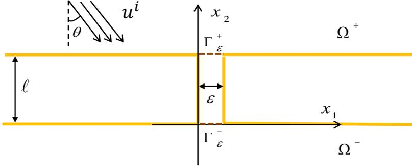
FIG. 1.1. *Geometry of the problem.* The slit  $S_\varepsilon$  has a rectangular shape of length  $\ell$  and width  $\varepsilon$  respectively. The domains above and below the perfect conductor slab are denoted as  $\Omega_+$  and  $\Omega_-$  respectively, and the domain exterior to the perfect conductor is denoted as  $\Omega_\varepsilon$ , which consists of  $S_\varepsilon$ ,  $\Omega_+$ , and  $\Omega_-$ .
