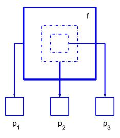
Figure 1: A diagram showing how the images  $\mathbf{p}_1$ ,  $\mathbf{p}_2$ , and  $\mathbf{p}_3$  of different resolutions are taken from part of the scene or the whole scene.
