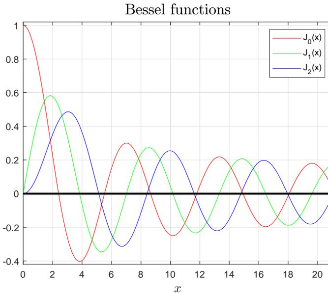
Before you start computing the roots, I would recommend plotting the Bessel functions  $J_n(x)$  versus  $x$  as I have done above. From the plot, you can easily visualize the behavior of the roots. To plot the Bessel functions, you can make use of the MATLAB function `integrate.m`.
