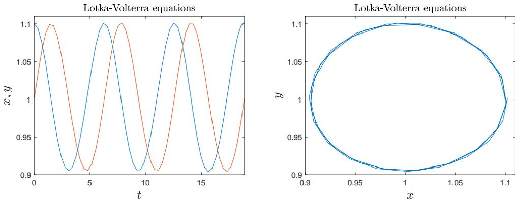
A careful inspection of the figures reveals two anomalies. First, in the plot of  $x$  and  $y$  versus  $t$ , there are not enough data points in the output for a smooth plot, particularly at the maxima and minima of the functions where the linear interpolation of the data is evident. Second, in the phase-space plot of  $y$  versus  $x$ , it is unclear whether the solution is exactly periodic since overlapping curves are evident.
