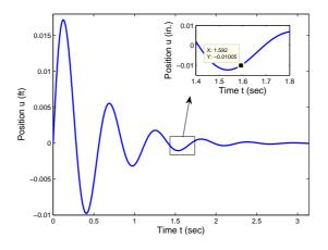
Suppose the mass first return to its equilibrium position at  $u(t_1) = 0$ , so  $t_1 = \frac{\pi}{2\sqrt{31}}$  sec. From the figure, we know  $\tau = 1.59$  sec. We note that the length 0.01 is in inch, that is 1/100 of a foot.
