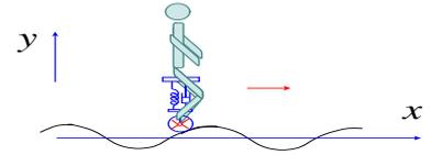
where  $y(t)$  is the displacement from equilibrium position,  $m = 300$  kg is the mass,  $k = 12000$  N/m the spring constant, and  $\gamma$  the damping constant. Note that the distance travelled in the  $x$ -direction after time  $t$  is  $x = vt$ .
