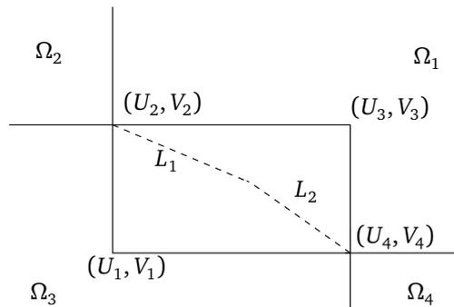
Figure 10: The delta-shock solution of the pressureless equations due to the interaction of vortex sheets. This figure is displayed in the self-similarity  $(x/t, y/t)$ -plane. The notation  $(U_i, V_i)$  denotes the coordinate  $(x/t, y/t) = (U_i, V_i)$ ,  $i = 1, 2, 3, 4$ . The dashed line denotes the support of delta-shocks.
