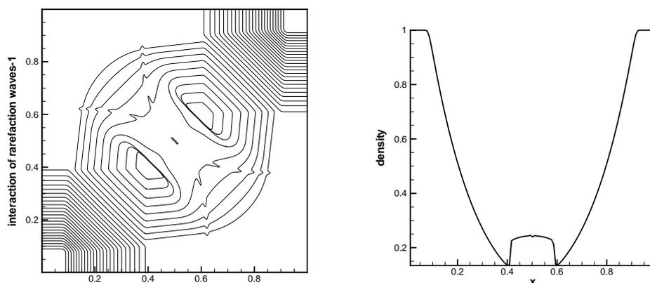
Figure 13: Interaction of planar rarefaction waves with initial condition Eq. (3.9).
