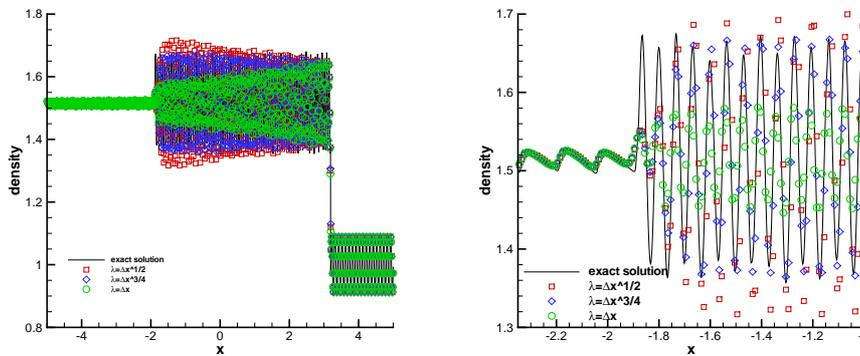
Figure 2: The density distribution and local enlargement of Titarev-Toro problem at  $t = 5$  for WENO-Z+ weights with  $\lambda = \Delta x^{1/2}, \Delta x^{3/4}$  and  $\Delta x$ .
