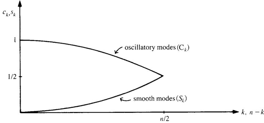
Figure 5.6: Damping factor for the two-grid correction operator  $TG$ , without relaxation, acting on the oscillatory modes with wavenumbers  $n - k$  (upper curve) and on the smooth modes with wavenumbers  $k$  (lower curve) for  $1 \leq k \leq \frac{n}{2}$ .
