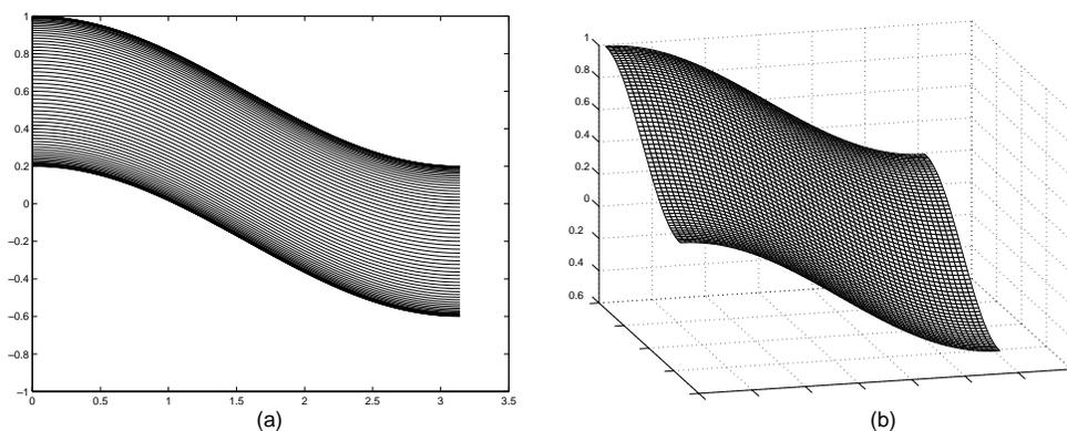
Figure 4.4: (a) Amplification factor,  $G(\theta_1, \theta_2)$ , for the weighted Jacobi method applied to the model problem in two dimensions, shown as individual curves of fixed  $\theta_1$  ( $\theta_1 = 0$  at the top and  $\theta_1 = \pi$  at the bottom). (b) Same amplification factor shown as a surface over the region  $[0, \pi] \times [0, \pi]$ . The picture is symmetric about both the  $\theta_1$ - and  $\theta_2$ -axes.
