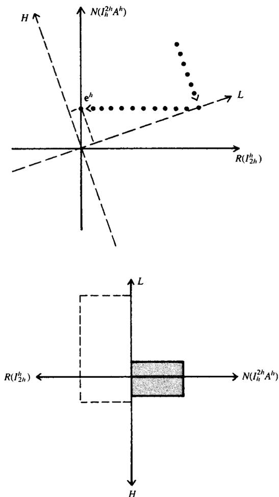
Figure 5.10: The top diagram shows the error after doing the remainder of the two-grid correction. All components in  $\mathcal{R}(I_{2h}^h)$  are eliminated as indicated by the projection onto the  $N$ -axis. The lower diagram shows the corresponding changes in the energy budget.
