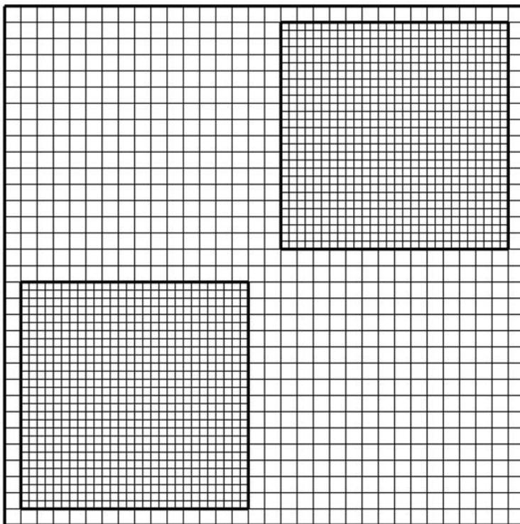
Figure 9.6: Aerial view of a composite grid based on a  $31 \times 31$  interior global grid of mesh size  $h = \frac{1}{32}$  and  $27 \times 27$  patches of mesh size  $\frac{h}{2} = \frac{1}{64}$  centered at  $(\frac{1}{4}, \frac{1}{4})$  and  $(\frac{3}{4}, \frac{3}{4})$ .
