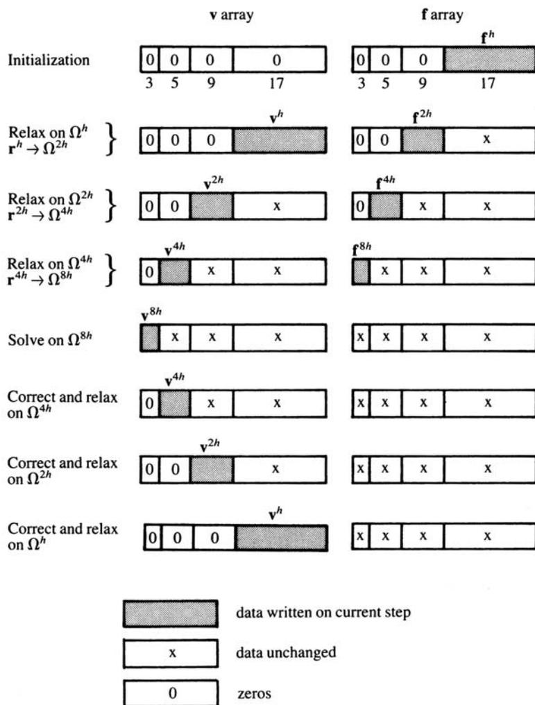
Figure 4.1: Illustration of the course of a four-level ( $n = 16$ ) V-cycle showing changes in the data arrays. The  $\mathbf{v}$  and  $\mathbf{f}$  arrays hold the solution vectors and right-side vectors, respectively, in the four grids.
