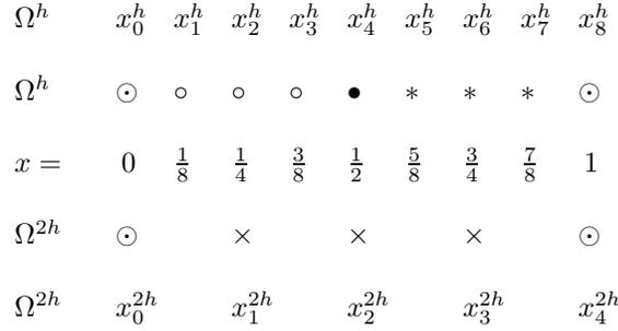
Figure 9.2: Local fine-grid points on  $\Omega^h$  are denoted by  $*$  and the interface point is denoted by  $\bullet$ . Computation at the remaining fine-grid points ( $\circ$ ) is eliminated. The coarse-grid points ( $\times$ ) comprise  $\Omega^{2h}$ , while  $\odot$  represents boundary points.
