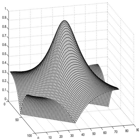
Figure 4.5: Amplification factor,  $|G(\theta_1, \theta_2)|$ , for the Gauss–Seidel method applied to the model problem in two dimensions, shown as a surface over the region  $[-\pi, \pi] \times [-\pi, \pi]$ .
