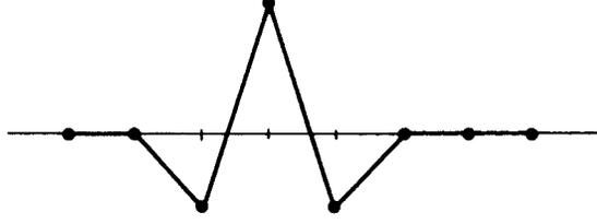
Figure 5.4: A typical basis vector of the null space of the full weighting operator  $N(I_{2h}^{2h})$ .
