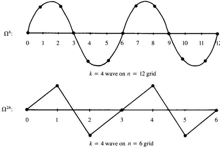
Figure 3.1: Wave with wavenumber  $k = 4$  on  $\Omega^h$  ( $n = 12$  points) projected onto  $\Omega^{2h}$  ( $n = 6$  points). The coarse grid “sees” a wave that is more oscillatory on the coarse grid than on the fine grid.
