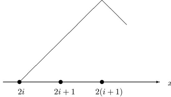
Figure 10.4: Cross-section of the grid along a line of constant  $y$  showing the coarse-grid points  $(2i, 2j)$  and  $(2(i+1), 2j)$  and the intermediate fine-grid point  $(2i+1, 2j)$ . The coarse-grid element is linear in  $x$  between the two coarse-grid points.
