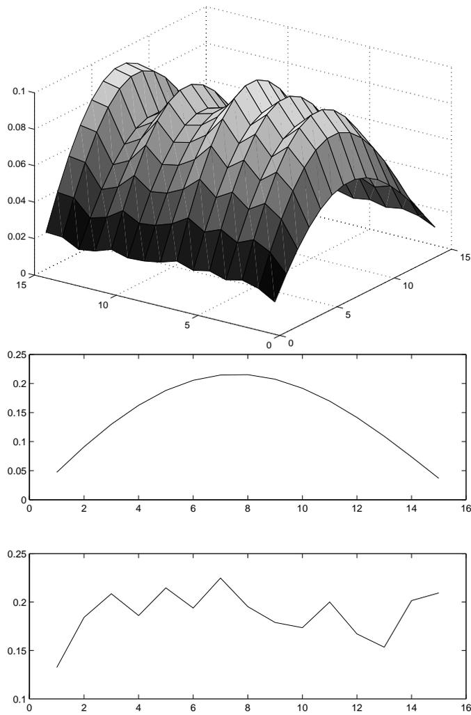
Figure 7.6: *Top: Error after 50 sweeps of pointwise Gauss-Seidel on the equation  $-u_{xx} - \epsilon u_{yy} = 0$ , beginning with a random initial guess. Middle: Error in the strongly coupled x-direction along a line of constant y. Bottom: Error along a line of constant x, in the weakly coupled y-direction.*
