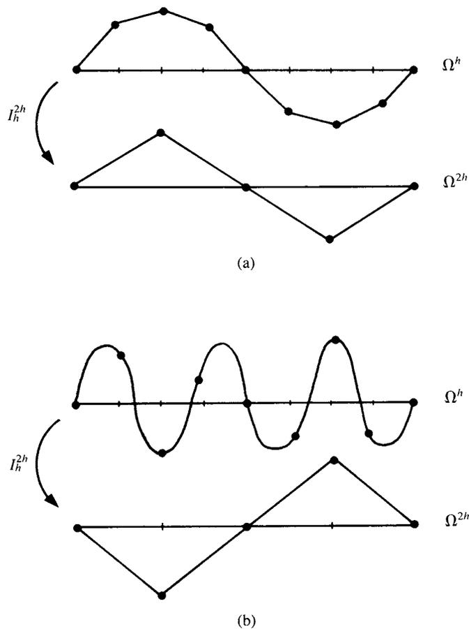
Figure 5.2: The full weighting operator  $I_h^{2h}$  acting on (a) a smooth mode of  $\Omega^h$  ( $k = 2$  and  $n = 8$ ) and (b) an oscillatory mode of  $\Omega^h$  ( $k = 6$  and  $n = 8$ ). In the first case, the result is a multiple of the  $k = 2$  mode on  $\Omega^{2h}$ . In the second case, the result is a multiple of the  $n - k = 2$  mode on  $\Omega^{2h}$ .
