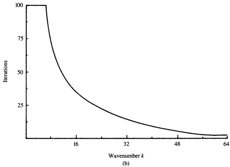
Figure 2.11: Gauss–Seidel iteration matrix applied to the model problem with  $n = 64$  points. The initial guesses consist of (a) the eigenvectors of the iteration matrix  $R_G$  with wavenumbers  $1 \leq k \leq 63$  and (b) the eigenvectors of  $A$  with wavenumbers  $1 \leq k \leq 63$ . The figure shows the number of iterations required to reduce the norm of the initial error by a factor of 100 for each initial guess.
