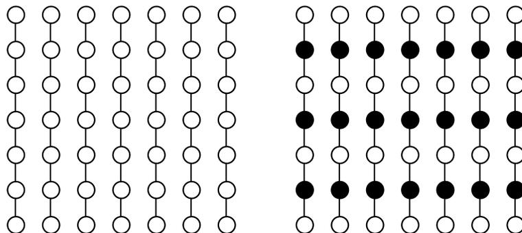
Figure 8.7: *Semi-coarsening produced for a stretched mesh (or anisotropic) problem. Shown on the left is the grid with only the strong dependencies indicated. On the right, the final coarsening is displayed.*
