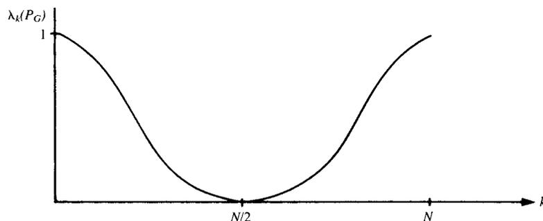
Figure 2.10: *Eigenvalues of the Gauss-Seidel iteration matrix. The eigenvalues  $\lambda_k = \cos^2\left(\frac{k\pi}{n}\right)$  are plotted as if  $k$  were a continuous variable on the interval  $0 \leq k \leq n$ .*
