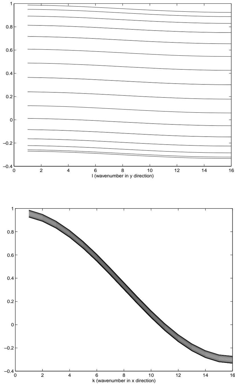
Figure 7.2: The upper plot shows the eigenvalues of the Jacobi iteration matrix, with  $\omega = \frac{2}{3}$ , along lines of constant  $k$  (wavenumber in the  $x$ -direction). The upper curve corresponds to  $k = 1$  and the lower curve to  $k = n = 16$ . The lower plot shows the same eigenvalues along lines of constant  $l$  (wavenumber in the  $y$ -direction). The small parameter in (7.14) is  $\epsilon = 0.05$ .
