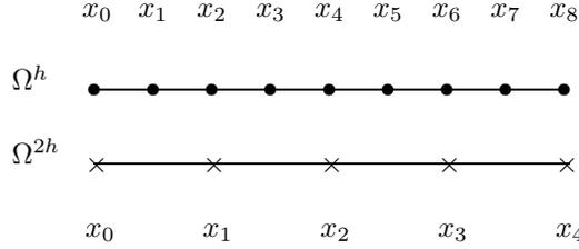
Figure 7.1: For the Neumann boundary condition case, the solution is unknown at the end points  $x_0$  and  $x_{n+1}$ , where  $n$  is an odd integer. The figure shows  $\Omega^h$  and  $\Omega^{2h}$  for the case  $n = 7$ .
