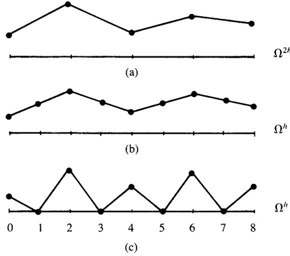
Figure 5.1: The action of  $A^h$  on the range of interpolation  $\mathcal{R}(I_{2h}^h)$ : (a) an arbitrary vector  $\mathbf{u}^{2h} \in \Omega^{2h}$ ; (b) the linear interpolant  $I_{2h}^h \mathbf{u}^{2h}$ ; and (c)  $A^h I_{2h}^h \mathbf{u}^{2h}$ , which is zero at the odd grid points on  $\Omega^h$ .
