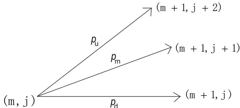
The  $(m, j)$ -node at the  $m^{\text{th}}$  time step and  $j^{\text{th}}$   $R^*$ -level moves to  $(m+1, j+2)$ ,  $(m+1, j+1)$  and  $(m+1, j)$  nodes with respective probabilities  $p_u$ ,  $p_m$  and  $p_d$  in the next time step.
