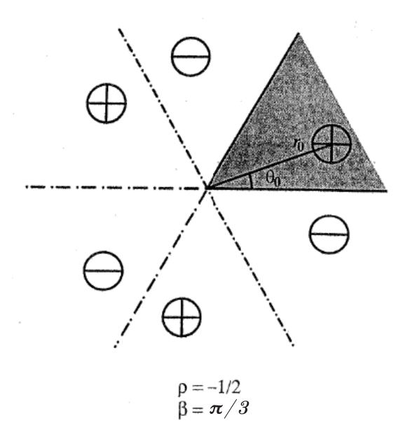
A method of images solution for the two-dimensional case.
