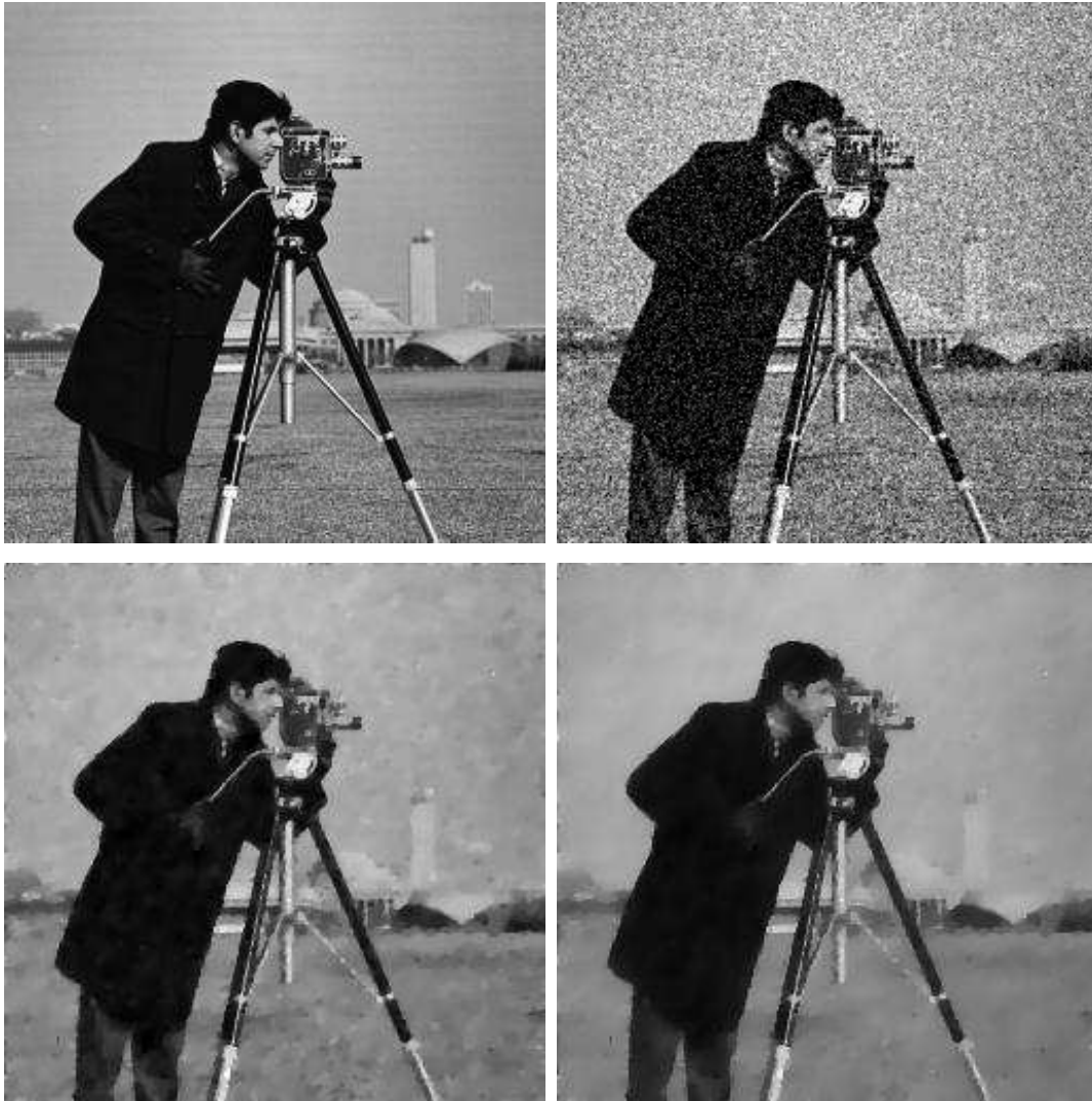
FIGURE 3. Some comparisons using artificial noise. The original image (upper-left) is added with Gaussian white noise (upper-right). The standard TV denoised image (lower-left) has more noisy residual than the wavelet TV denoised image (lower-right). Both are obtained with same number of iterations.
