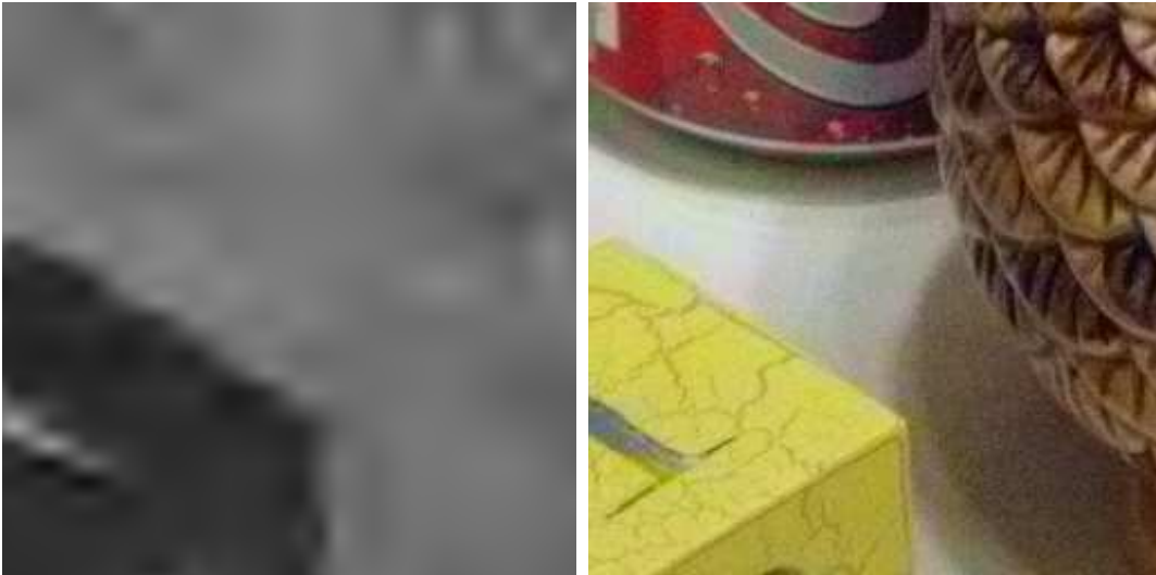
FIGURE 6. The other chrominance channel Cb (left) is also severely blurred by wavelet thresholding. While the re-composed color image (right) after blurring the CrCb channels seems to be a reasonable approximation to the original one.
